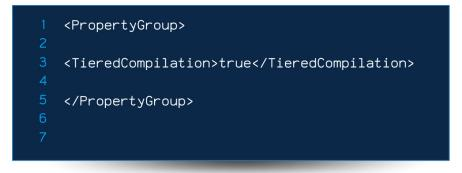
While tiered compilation offers many benefits, avoid it in situations where the recompilation of hot methods consumes additional CPU resources, as that could impact performance temporarily. That means applications with very short run times or those that are highly sensitive to CPU usage spikes during their startup phase might not benefit as much from this feature.
